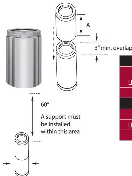
Used in combination with straight insulated lengths, the adjustable length makes it possible to fit a length perfectly, either vertically, horizontally, or at an angle.
