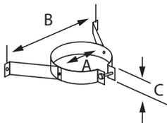
Use to provide lateral stability when chimney runs up an interior or exterior wall. Adjustable arms slide in or out to set required clearances. Adjustable collar works with 5", 6", 7", or 8" pipe.
