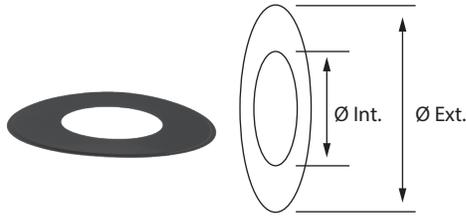
The optional decorative Trim Collar can be used to help provide a professional finish around the chimney when passing through a non-combustible wall.
