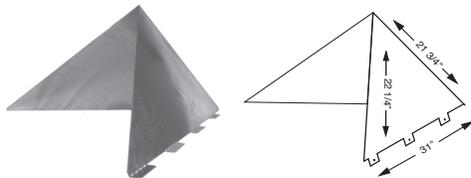
Ships flat, and folds easily on the job site. Includes 8 fastening flanges (4 on each side) for mounting. Made with heavy 14 gauge galvanized steel.
