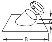
Galvanized Adjustable Roof Flashing. Choose from three different versions to match roof pitch. Storm collar is included.
