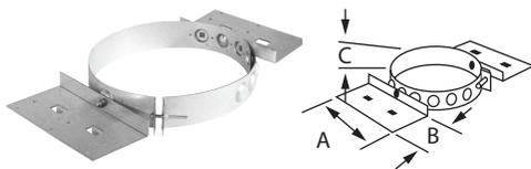
The roof support is versatile. A universal collar allows it to fit 5", 6", 7" and 8" chimney. It is typically used to support a chimney at the roof-deck. The mounting brackets easily adjust to suit any pitch. It can also be used as a re-support when placed upon a floor or mounted to a ceiling; or as offset support. Please refer to instructions for more details.
