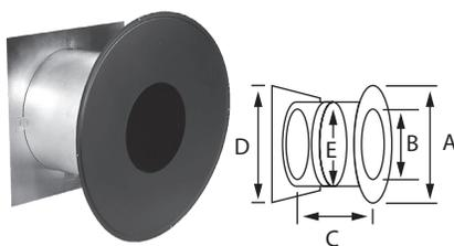
Designed to protect surrounding combustible materials when a chimney passes through a wall. Thimble works with wall thicknesses from 7" up to 12-1/2". Can be trimmed for use with thinner walls. Includes painted Decorative Collar for interior finish. Insulated to prevent heat loss or cold air intrusion.
