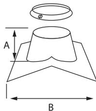
Galvanized Peak Roof Flashing. Choose from two different versions to match roof pitch. Storm collar included.
