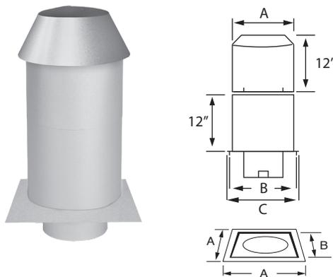
Two-piece overlapping design adjusts from 12" up to 22" height to accommodate deeper levels of insulation. Part is factory-insulated and includes both the base plate and collar as shown.
