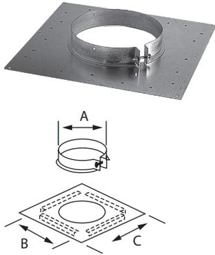
Use to support the chimney on a slab, floor, or joist. It includes a tightening collar that locks around the chimney and is secured by self-tapping screws (included). The collar rests on a horizontal plate screwed or nailed to the floor or slab. It can also serve as an intermediate support. Refer to chart for load bearing capacity.
