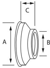
Use this optional part if desired to conceal 5" projection of horizontal chimney section within dwelling. Must be used in combination with flue extension.
