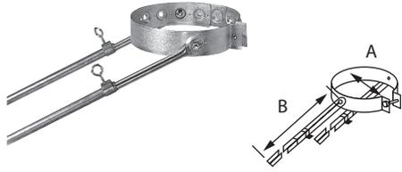
Required to stabilize chimney against wind-loading when 5 feet or more extends above the roof-line. Adjustable collar works with 5", 6", 7", or 8" pipe. Brace arms are adjustable from 60" up to 115".
