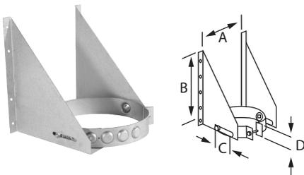
Use to support the chimney on a vertical wall. The triangular plates allow for a 2 3/4" adjustment of the support to the vertical surface. This support can also be used as a wall support above the insulated tee or as a support for an offset elbow. Refer to chart for load bearing capacity. In shorter chimney stack applications, the Wall-Support can also be used in place of a Tee Support. Universal design works with 5", 6", 7", or 8" pipe diameters.
