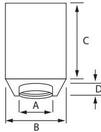
Support for use with vaulted or cathedral ceilings. 6" version fits within 12" x 12" frame. Larger 7" and 8" versions will fit within frame between 16"-on-centre construction. Includes two-piece adjustable black finish trim. Integrated adapter accepts both single-wall or double-wall stovepipe.
