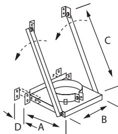
Use to support insulated tee on though-wall chimney installation. For installation versatility and convenience, tee can be placed above or below the support. Can also be used as a wall support or re-support. Adjustable arms and sliding base plate are factory-set to ensure minimum clearance of 2". Allows for 2" - 7" clearance to combustibles.
