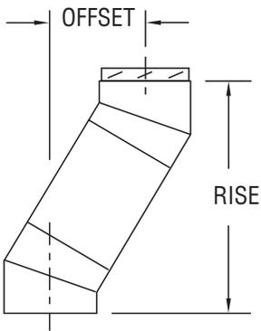
Use to determine the lengths required for an installation. Determine the offset required in view of the obstacles that must be avoided. Refer to the offset/rise chart to determine the elbows required as well as the insulated lengths needed. Check the corresponding offset height dimensions.
