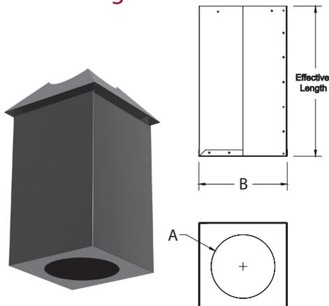
Use when insulated chimney passes up through a ceiling penetration from below. Suited for flat, vaulted, or cathedral applications. Integrated Firestop on bottom. Top can serve as an Attic Radiation Shield where required.
