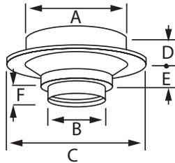
Same as above except collar is fixed; not removable. Integrated adapter accepts either single-wall or double-wall stovepipe.
