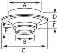
Round Finishing Support for use on flat ceiling. 6" diameter only. Fits within 12-3/8" x 12-3/8" frame. Integrated adapter accepts either singlewall or double-wall stovepipe. Removable trim collar allows collar to be fastened in place after finish of ceiling is completed.
