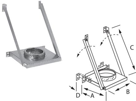
Use to support insulated tee on though-wall chimney installation. Access for inspection and service is incorporated from the underside of this support. Adjustable arms and sliding base plate are factory-set to ensure minimum clearance of 2". Allows for 2" - 7" clearance to combustibles.
