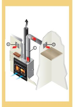
Osburn also offers you another way to distribute excess heat into your home with the help of a hot air gravity kit.
