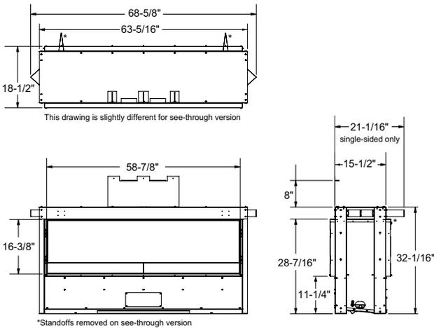
NOTE: Gas Connection/Electrical connections if using optional Hardwire Kit are located on left hand side of appliance.
