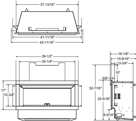
NOTE: Gas Connection/Electrical connections if using optional Hardwire Kit are located on left hand side of appliance.
